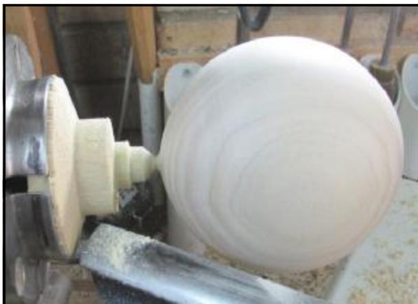
Now reduce the diameter of the main spigot to the "16 Side" dimension, and on the single remaining corner, repeat the process detailed in the previous paragraph using the "16 Side Trim" dimension.
