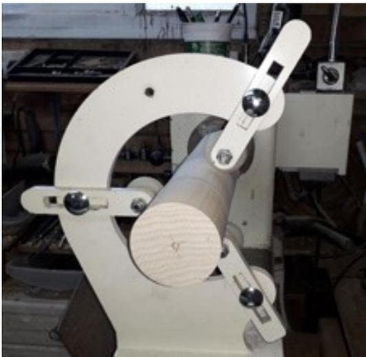
**On a bigger bottle it is almost a pre-requisite that you use a steady rest to support the blank as shown here.**
