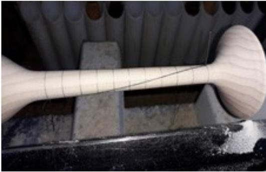
Put your first mark at the top, just below the bell section, then add extra marks all the way down the tapered neck. I have tried 10mm sections on a small bottle, and on bigger pieces, try starting at 10mm, and increase the width of each segment by 1mm as you make your way down the neck. Both work well, but keep them small on a small bottle.
