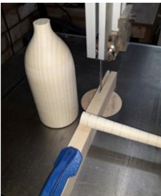
Clamp a batten onto the bandsaw table. It needs to have a long slot in it where the blade will run.
