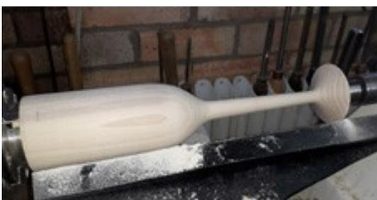
**Cut the bottle to shape and sand it well. You need to get a fine smooth taper on the neck section. On big bottles aim for 3/4" tapering down to 1/2", and on smaller bottles aim for 5/8" tapering down to 3/8".**
