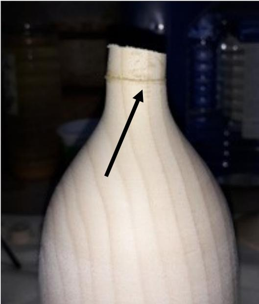
Having sanded the first disc, glue it to the top of the bottle. Use the original marks as an alignment guide, BUT, pay close attention to the grain patterns, it is most important that they align correctly.
