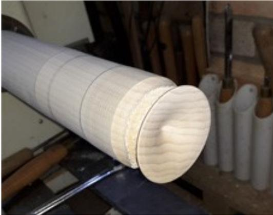
**The next stage is to hollow the free end, a bit like the bell end of a trumpet. On a small bottle you can do this by making very fine cuts with a spindle gouge after pulling the tail stock away.**
