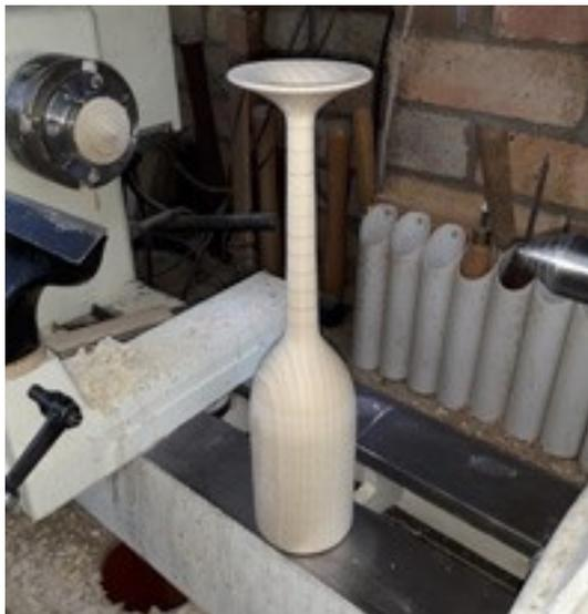
Part off at the base, having rounded off and sanded the bottom corner, just as you would see on a real bottle.
