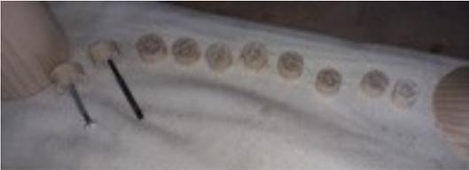
Each of the segments has had a small hole drilled through the centre. Find something to fit in the hole so that you can hold the piece while sanding.
