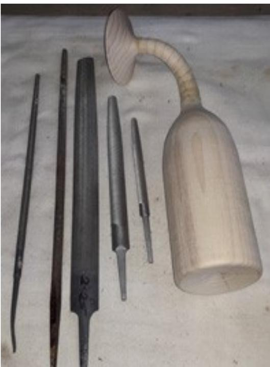
Having assembled the piece, set it aside for a day or so, and then attack it with files and sandpaper. I find that round and half-round files work best. Work on it until you cannot feel any irregularity in either the line or the feel of the neck.
