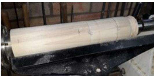
**Mark where you are eventually going to part the piece off, about half an inch from the chuck. Also, mark where the shoulder of the bottle is going to be. I normally aim this to be about an inch below centre.**
