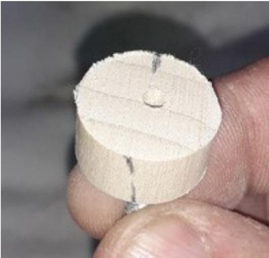
Sand the top surface of the un-necked bottle. It needs to slope downward towards the edge mark.
