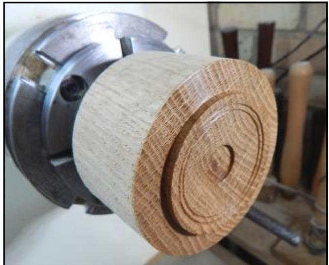
Put the lid section in the chuck, true up, and cut a small spigot section on the open face using a spindle gouge and skew. This spigot needs to be a good tight fit on the hollowed box section. When you are happy with the fit, hollow the centre section of the lid, add decoration, and finally, sand, seal and polish to your satisfaction, taking great care NOT to lose that tight fit on the base section.
