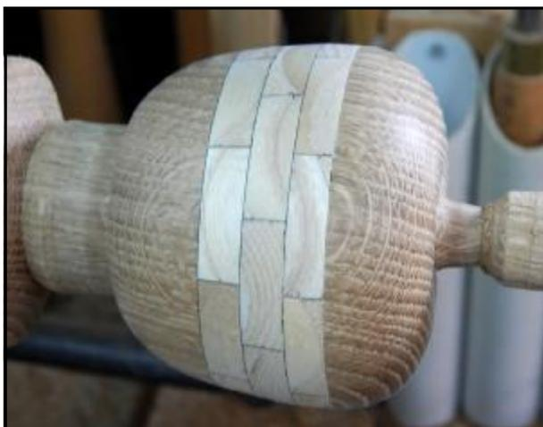
With the base section back in the chuck, fit the lid and hold it in place with a slim live centre, cut the outer profile of your apple, reaching as far as you can round to the upper and lower holding points. Remove the tailstock support and gently turn away the last bit on the lid section leaving a nice apple shaped
