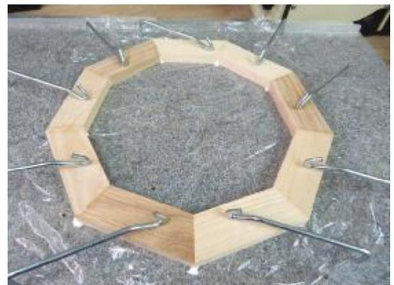
the invention of "The Spider Board", a piece of 40mm kitchen worktop and a set of re-purposed tent pegs. Bent so they can be pushed into pre-drilled holes, they have a natural spring action which will lock themselves in place until you see fit to remove them. When in use, the board gets covered with either cling film or aluminium foil to prevent the work sticking.
