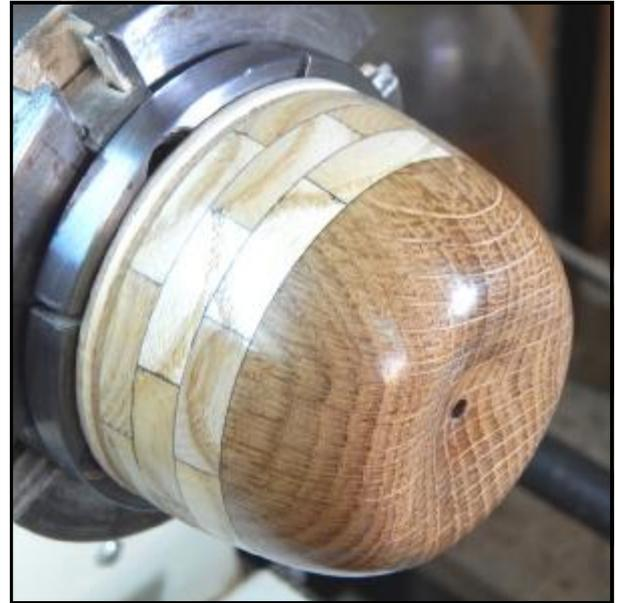
finish so that the lid has a "NASA" fit (lift off). With this type of box, the apple stalk will always be used as the handle, so the lid must not be a tight fit.
