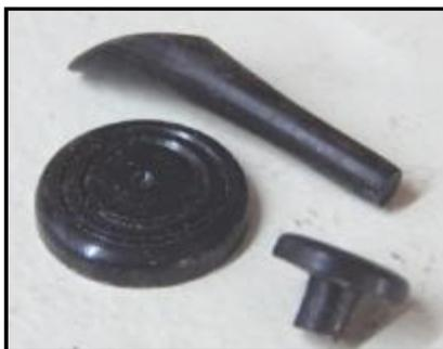
Using bits of African Blackwood, make a pip to fit in the bottom, a decorative insert to fit in the inside of the lid, and a stalk for the top of the lid. Drill a 3.5mm hole in the centre of the lid to take the stalk, again, taking great care to NOT drill through to the interior. Glue the Blackwood pieces into the lid section using your favoured brand of adhesive.
