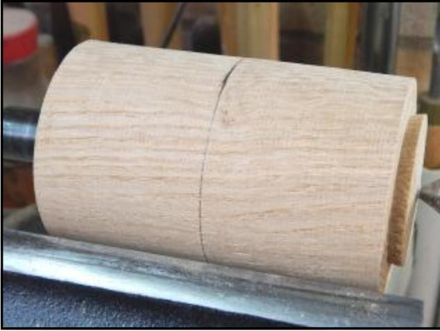
fashion), round off with a spindle roughing gouge and add a dovetail spigot at both ends. With the blank held in 50mm chuck jaws I part off a section, just right of
