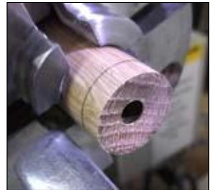
Mount the blocks back on the mandrel and turn both down to the finished size and shape. Make sure the barrel ends are turned down to the same diameter as the spacer bushes.
