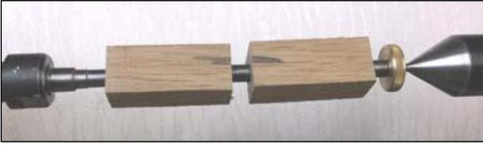
and sets in the presence of moisture, an inherent constituent of wood. Also, glue goes in the hole which is a lot less messy and no pre-cleaning is needed. Before inserting a brass tube into a glued hole, insert a potato plug into both ends of the tube, it will make the cleaning up stage a lot easier. Set the glued blocks aside for 4 or 5 hours to ensure the glue is set. Clean any glue overspill from the blocks and tubes, use a 1mm undersize drill to help with this.
