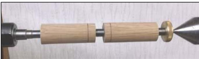
through at about 400 rpm using hand pressure on the tailstock to advance the work.
