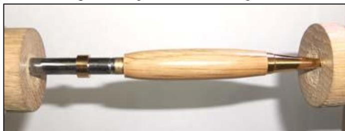
insertion to get the correct protrusion of the biro point through the bottom of the barrel. **DO NOT** insert the twister too far, once inserted you will never get it out. Using a wooden plug and the metal bracket, fit the cap and pocket clip into the top of
