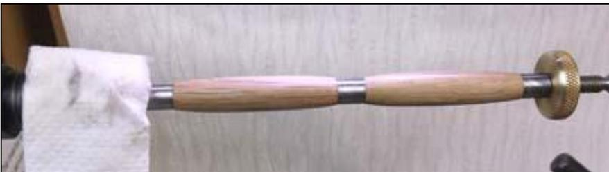
Wooden pens need to be sanded from 240 grit to about 600 grit. After sanding a set of wood blanks you should clean the mandrel bushes with
