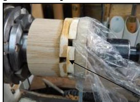
Repeat the process with 6 60 degree segments on the other side of the wheel. Make sure the gaps in the 1st ring of segments are centred on the edges of alternate segments in the 2nd ring as shown here.
