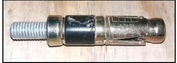
When designing this project, I paid a visit to my local DIY store and bought an M12 cavity bolt. This has an overall diameter which is very close to 20mm, a very good
