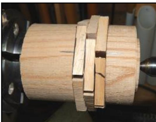
From this point on, the making of the apple is nothing remarkable. For safety, having mounted the larger section of the blank in the chuck, I normally provide tailstock support with a live centre, just until I am confident that the blank is in balance, and it is all holding together.
