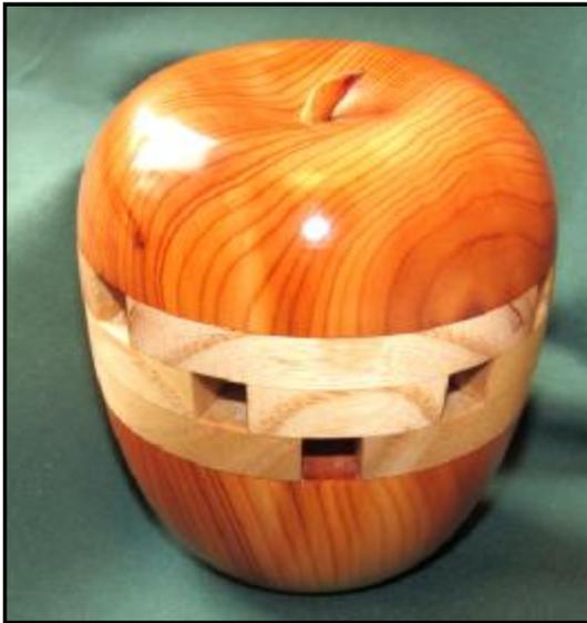
fit in the apple base. I disregarded the central bolt and replaced it with a short length of 12mm studding. With the studding mounted in the chuck you can then use the expanding section to re-mount the apple and finish turning it. Afterwards you should repeat the sanding and polishing.
