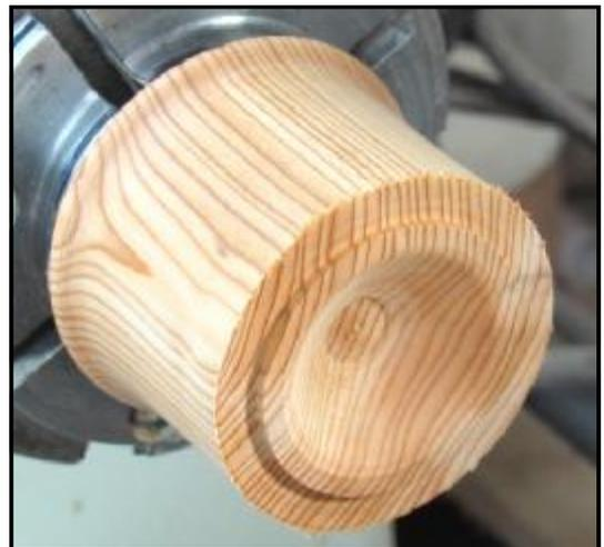
Trim the outer diameter of the blank down to 55mm, and leaving a 3mm skirt, taper the exterior of the lid section back towards the chuck with a smooth curve. The
