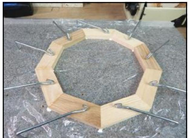
The basic process here is to lay down a sheet of cling film to work on followed by the set of segments (without glue), each being held in place with its own clip. Latterly I have used tinfoil, it is much easier to handle and just as effective. You should work with care, ensuring the joints are tight. You might need to fine tune the position or shape of some to get the last piece to fit correctly.
