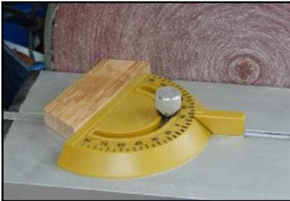
Having cut a set of segments to the defined size, sand ONE end of each segment on the disc sander, having previously gone to great lengths to set it's mitre fence correctly also (set it by testing the wood, NOT the fence). The only result which is acceptable here is a base angle of 70 degrees, plus or minus NOTHING. Also worth noting here is the importance of having the table set accurately (without flex) so that you sand at 90 degrees. Again, measure the angle on the wood, not the table.
