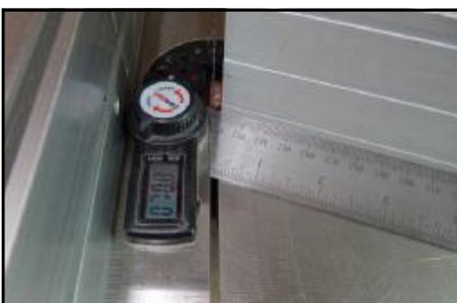
Stage one of the build process is to set the mitre fence on the bandsaw VERY ACCURATELY, so as to cut timber at the correct base angle.
