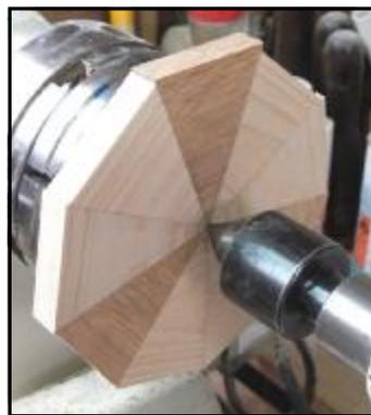
Make a sacrificial mount to hold in the chuck and use a sharp bowl gouge to cut a clean flat surface on the outside face. Use an awl to lightly mark the exact centre of your base ring, glue the face of the sacrificial chuck and hold the base ring in place with a live centre in the tail stock until the glue has gone off.
