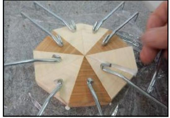
Only when you are happy with the layout do you start gluing. If you are working with an odd number of segments, remove one piece and apply glue to one edge only. Continue by removing alternate pieces, one at a time, applying glue to both edges and then clipping them back into place in the circle. After about an hour you can remove the ring from the spider board and move on to the next layer.
