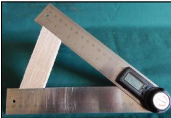
Having sanded the first end of each segment correct with respect to the LONG edge of the timber, all that remains is to sand the second end to 40 degrees with respect to the first. This is all very easy when you have a tool which will measure angles for you with good repeatable accuracy to within 1/10th of a degree.
